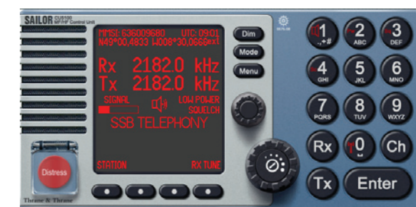
MF/HF radio station with DSC and Radiotelex SAILOR CU5100
