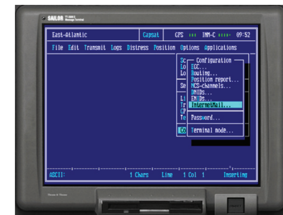
Inmarsat mini-C GMDSS SES SAILOR TT-3000E with internal GPS receiver and Remote Alarm/ Distress Box SAILOR TT-3043CP
